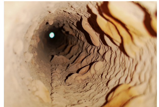
Limescale build-up inside lavatory pipes
