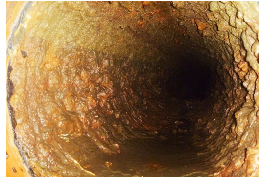
Limescale build-up inside lavatory pipes
